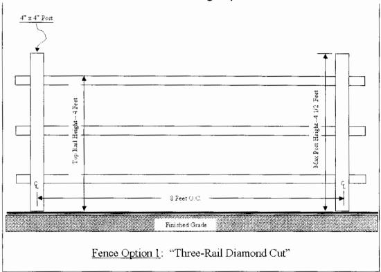
Note: Dimensions shown are NOT absolute. Please refer to the sections above for exact board width and spacing.
